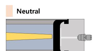
The disc does not contact the seat, resulting in low torque and reduce d actuator size
