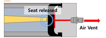
pneumatic signal fail, the air exhaust urgently within 0.5 seconds
